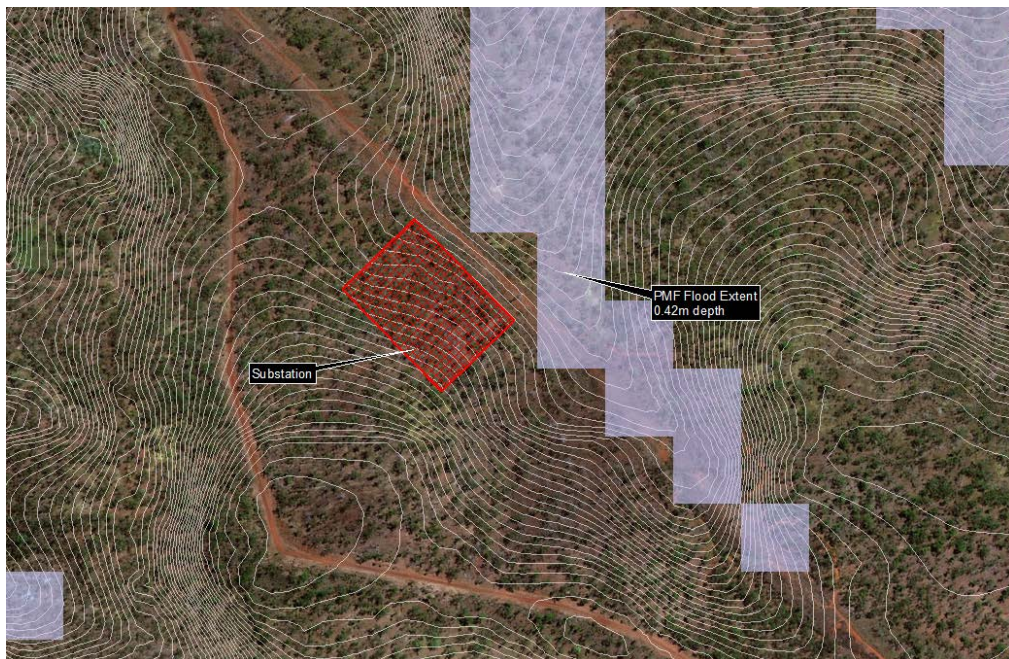
Figure 3 Mount Fox substation showing the flood extents for the PMF flood event
