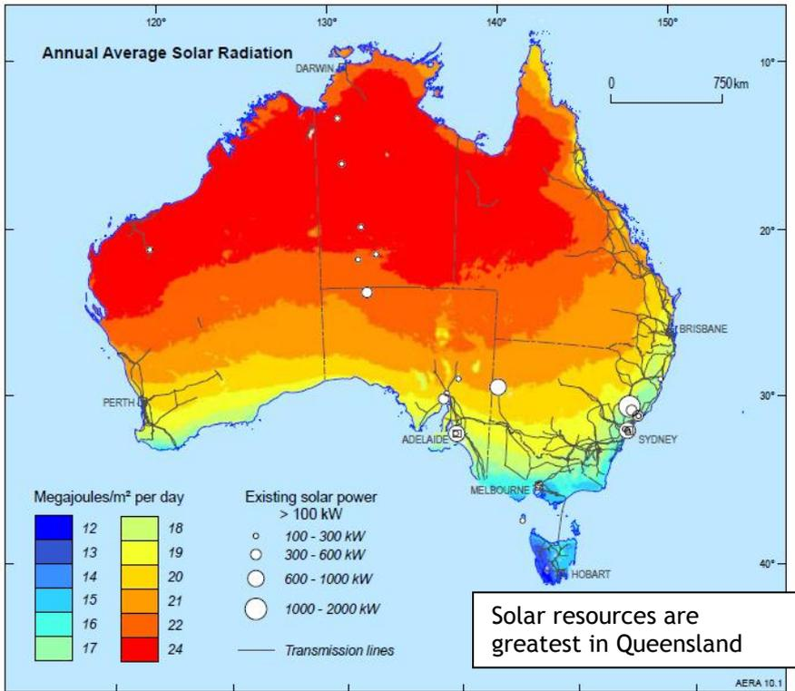
Figure 10.1 Annual average solar radiation (in MJ/m<sup>2</sup>) and currently installed solar power stations with a capacity of more than 10 kW
