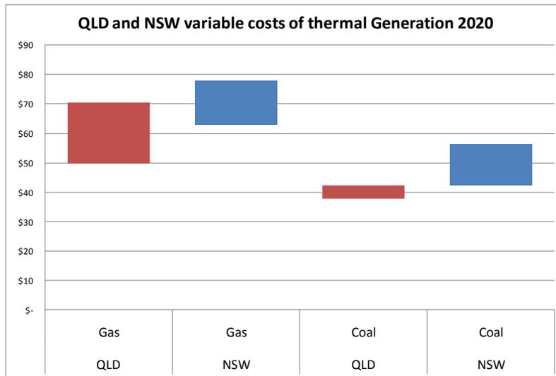
The chart indicates that coal fired plant in New South Wales and Queensland is often cheaper than combined cycle gas turbine (CCGT) plant and that Queensland coal fired plant tends to be cheaper than New South Wales coal plant, largely due to lower Queensland coal costs.
