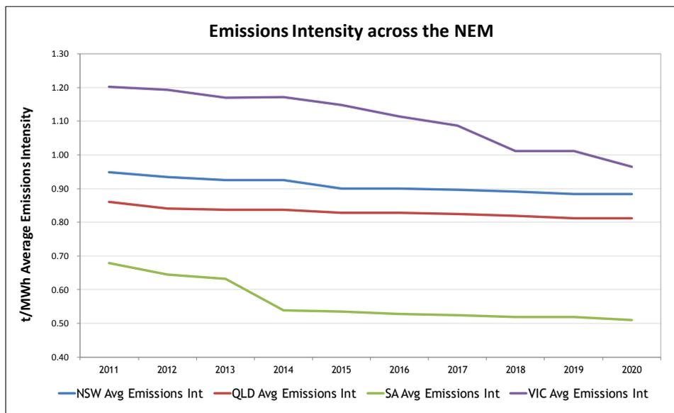
Generation in Queensland has a lower average emissions intensity (tonnes of carbon per MWh of energy produced) owing to the higher levels of gas and more efficient coal generation compared to New South Wales and Victoria. By way of comparison, South Australia has the lowest emissions intensity level of these four NEM states, due to a high proportion of wind and gas generation.
