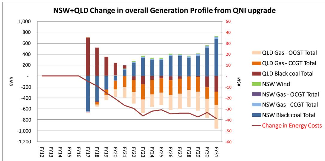
The graph shows that, with a 600MW upgrade on the interconnector, Queensland coal-fired plant displaces New South Wales coal-fired plant. This occurs initially at off-peak times and then gradually extends in the peak periods also. The key switch occurs in the 2021 financial year, when New South Wales coal-fired plant displaces the more expensive Queensland CCGT and OCGT capacity.
