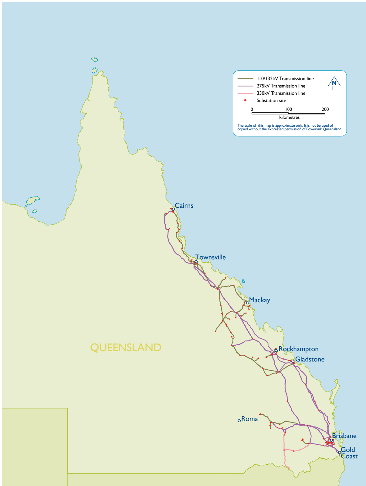
Figure 9.1 Existing Powerlink Queensland transmission network June 2017
