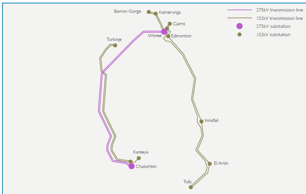
Figure 2.1: Far North zone transmission network
