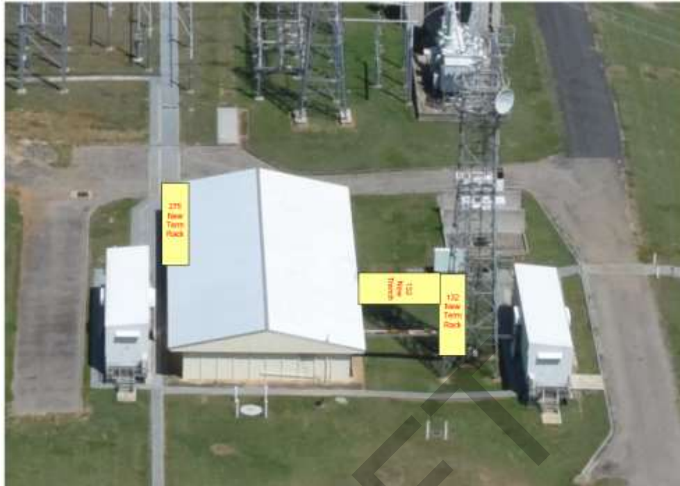
132kV/275kV Woolooga Substation proposed termination rack locations
