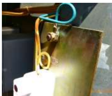
Figure 13: Wiring UV damages
