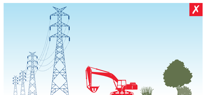
Operating mobile plant such as a tractor that breaches the overhead statutory clearance distances. Undertaking any activity that may intrude upon the regulated safety exclusion zone. Climbing a transmission tower.
