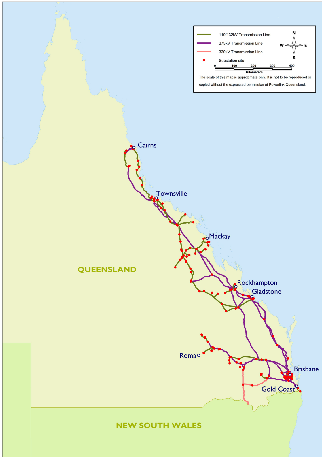
Figure 11.1 Existing Powerlink Queensland transmission network October 2021
