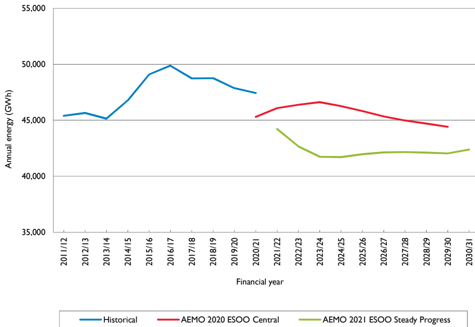
Figure 3.3 Comparison of AEMO's 2020 ESOO Central scenario delivered energy forecast with the 2021 ESOO Steady Progress scenario (I)
