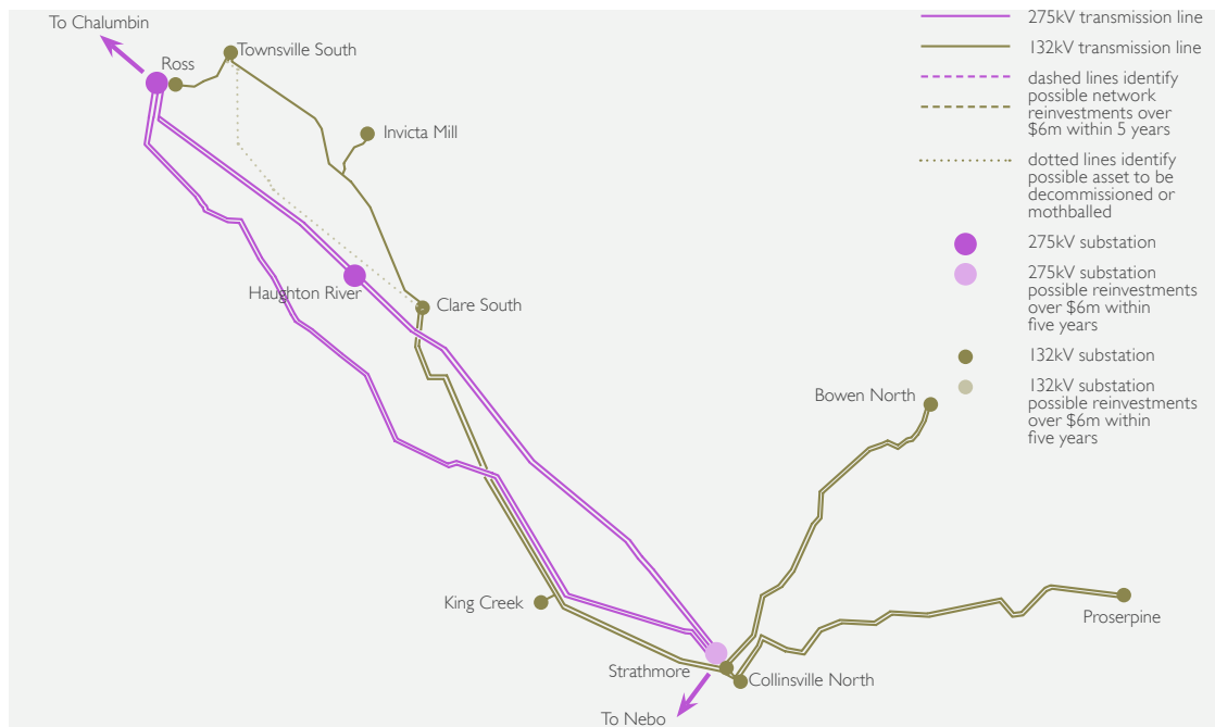
Figure 6.6 Southern Ross zone transmission network
