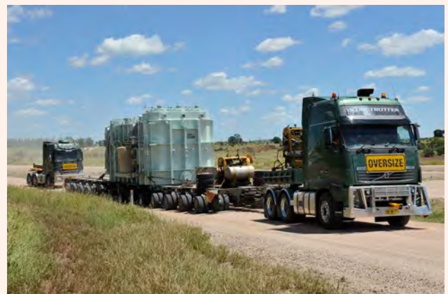
4. Heavy equipment such as high voltage transformers may be delivered at this time. Because of the very large size and weight of the transformers, delivery is often completed early or late in the day when there is less traffic on the road.
