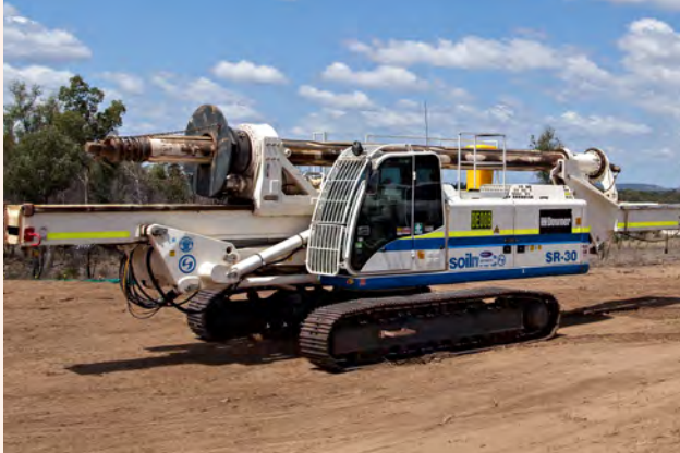
Boring machine Makes holes for foundations.
