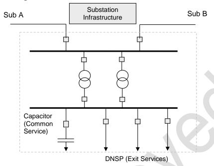
Step 1: The branches are Sub A, Sub B, DNSP1, DNSP2, DNSP3, Tie Transformer 1, Tie Transformer 2 and PCS.
