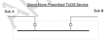
Step 3.2: The stand-alone arrangement for the provision of *prescribed common transmission services* to an equivalent standard is shown below and consists of 3 circuit breakers.
