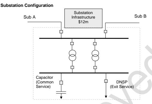
Step 1: The branches are Sub A, Sub B, DNSP, Tie Transformer 1, Tie Transformer 2 and *Prescribed Common Service*.
