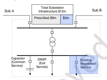
Step 1: The branches are Sub A, Sub B, DNSP, Tie Transformer, *Prescribed Common Service* and an existing negotiated service.
