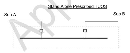
Step 3.2: The stand-alone arrangement for the provision of *prescribed common transmission* services to an equivalent standard is shown below and consists of 3 circuit breakers.
