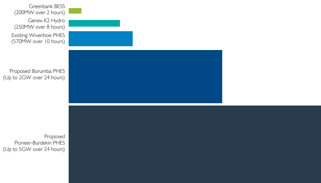
Figure 2.2 Relative energy storage capacities of PHES and BESS
