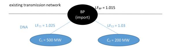
This is a load-only terminal *DNA* connected to the existing transmission network, so the only calculation required relates to the estimated losses calculated using the process outlined in <u>Case 1</u> above.
