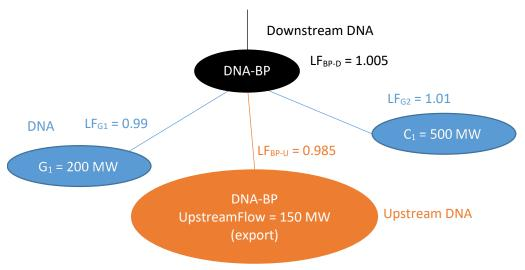
This *DNA* contains a mix of generation and load assets and has a downstream *DNA*, so the calculations required are estimated losses and downstream flows using the process outlined in Case 4 above.<sup>1</sup>
