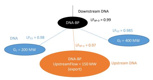
This *DNA* contains only generation assets, an exporting upstream *DNA* and a downstream *DNA*, so the calculations required are estimated losses and downstream flows using the process outlined in Case 3.
