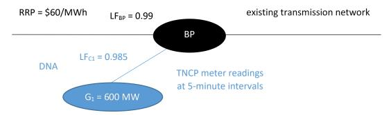
Intuitively, the estimated losses over the *DNA* reflect the difference in estimated energy at the *regional reference node* based on the hypothetical situation where the asset was located at the *boundary point* or *DNA boundary point*. In the example above:
