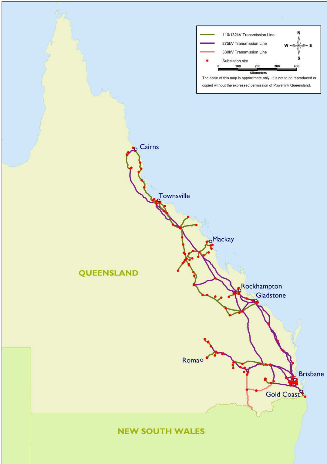
Figure 9.1 Existing Powerlink Queensland transmission network October 2023
