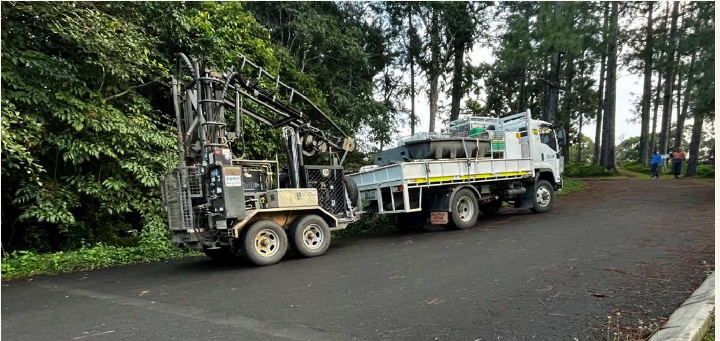
Example of drilling rig to be used during geotechnical investigations.
