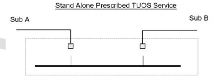
Step <u>3.24</u>: The stand-alone arrangement for the provision of *prescribed common transmission services* to an equivalent standard is shown below and consists of 3 circuit breakers.
