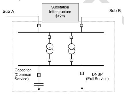
Step 1: The branches are Sub A, Sub B, DNSP, Tie Transformer 1, Tie Transformer 2 and Prescribed Common Service.
