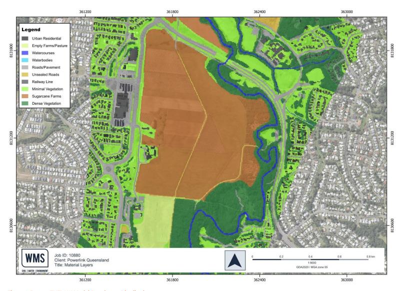
Figure 2-5 TUFLOW Model Roughness Distribution
