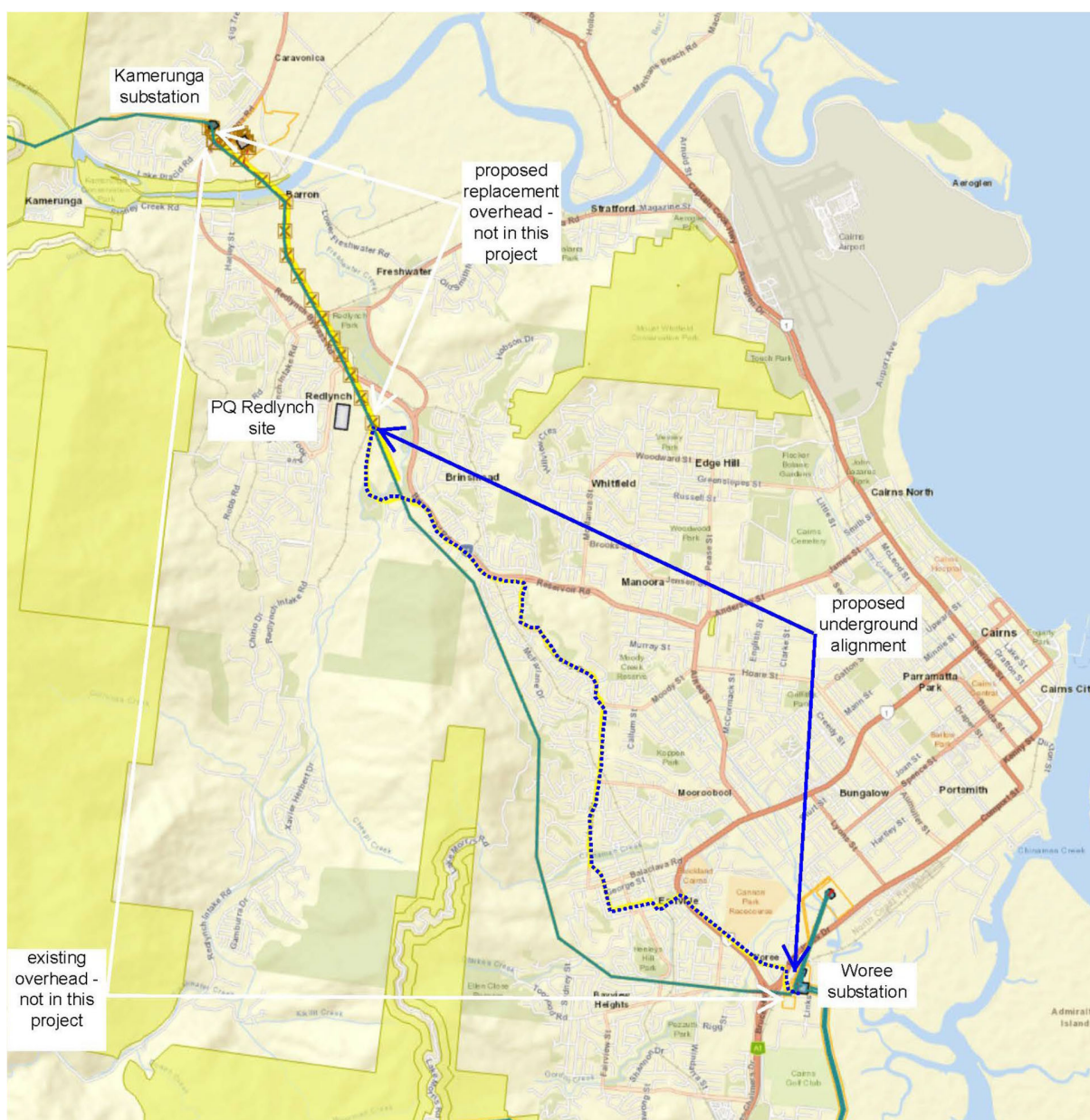
Figure 2 Map showing the existing overhead powerline and proposed underground cable
