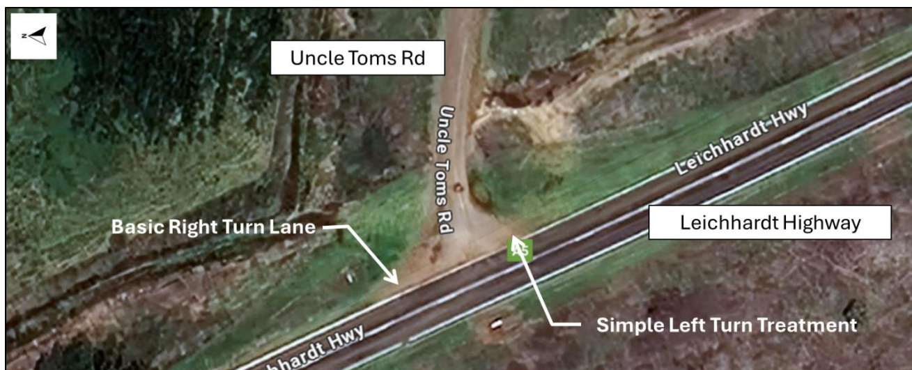
Figure 3.6 Leichhardt Highway / Uncle Toms Road intersection
