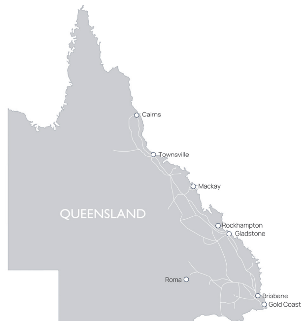
Figure 1: Queensland's electricity transmission network
