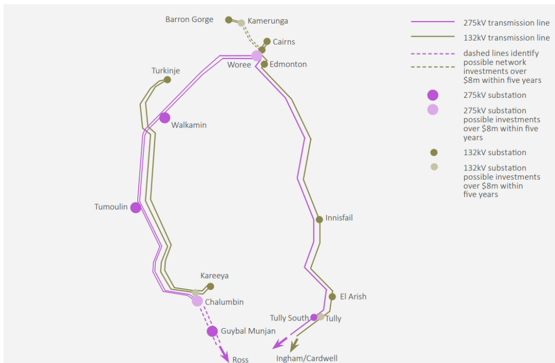
Figure 2.1: Far North zone transmission network
